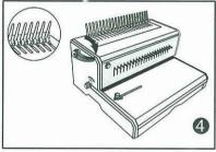
4. Move the plastic ring pulling handle ahead . and open the plastic ring .
