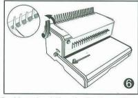
Move back the plastic ring pulling handle .close the plastic ring .and take out the documents. Finally turn off .
