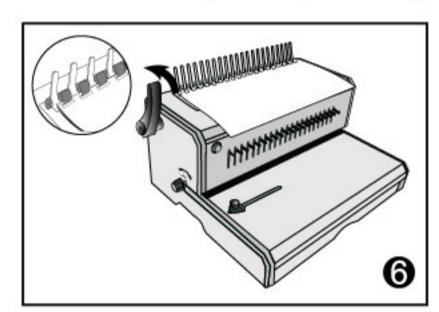
6. Move back the plastic ring pulling handle .close the plastic ring .and take out the documents. Finally turn off .
